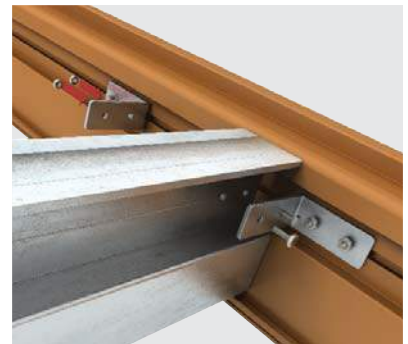
Fix rafters to ringbeam
