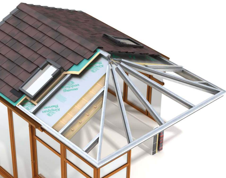
Guardian warm roof construction
