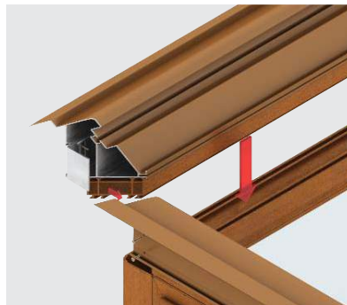
Fix ringbeam to existing windows
